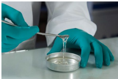
API powder dispersed into liquid PGS resin
