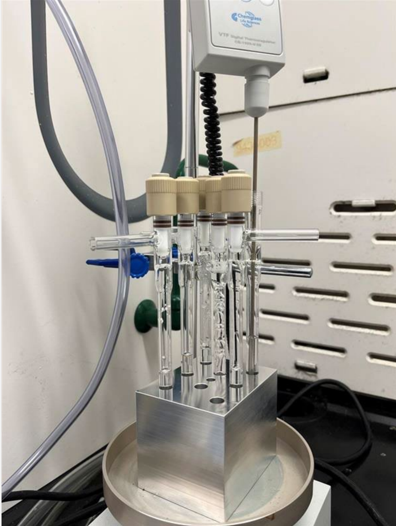
Figure 2. API-loaded PGSU rods were digested in 6 N HCl for 48 hrs at 110 °C. Samples were analyzed using LC-MS for cross-reactivity and to quantify the drug loading
