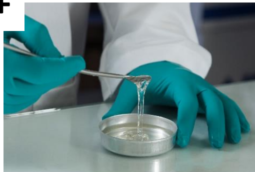
API powder dispersed into liquid PGS resin
