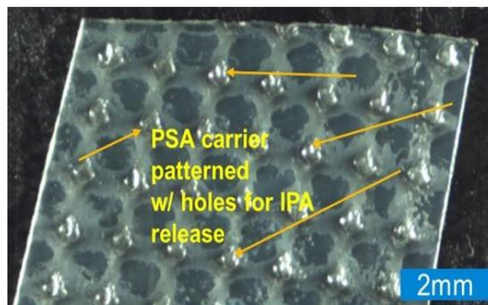
Figure 6 shows the Material A perforations on the PSA carrier film. These are through-holes that allow the isopropyl alcohol (IPA) swipe to percolate solvent through the bulk PSA film to the skin-adhesive interface.
